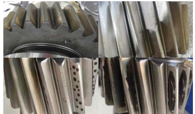
Fig. 5. (a) Healthy, (b) tooth fracture, (c) pitting, (d) spalling.
